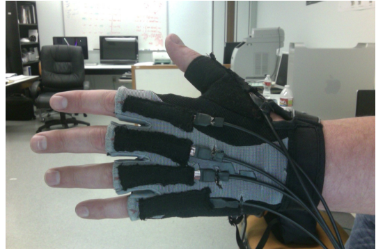
Fig. 4. Bend Sensors mounted on a glove
